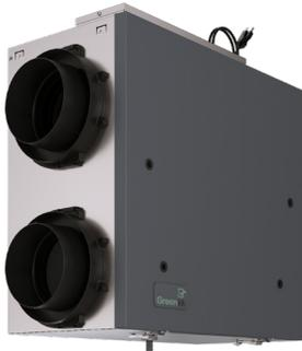
Greentek's PREMIER 2.0E is an Energy Recovery Ventilator designed for higher static pressure applications. The unit brings a continuous supply of fresh air into a home while exhausting an equal amount of contaminated air. The energy recovery core at the center of the unit transfers heat and moisture from incoming air to the outgoing air that was cooled and dried by the building's air conditioner.
